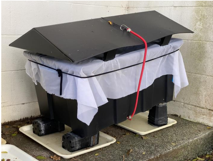
Figure 2. Raised lids were constructed and put on the bins to increase air flow within the bins (intended for bioconversion of grape marc by mealworms). A fine-mesh cloth was placed over the top of the bin to prevent access by organisms other than mealworms. Bungee cords were used to secure the lid against the wind.
