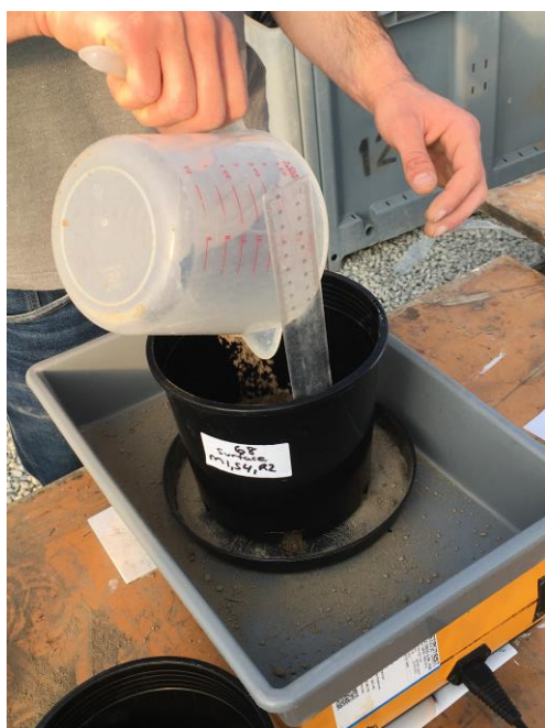
Figure 1. Pots being packed with soil on 24 June using electronic scales and ruler to pack the soil in two layers by weight and depth.
