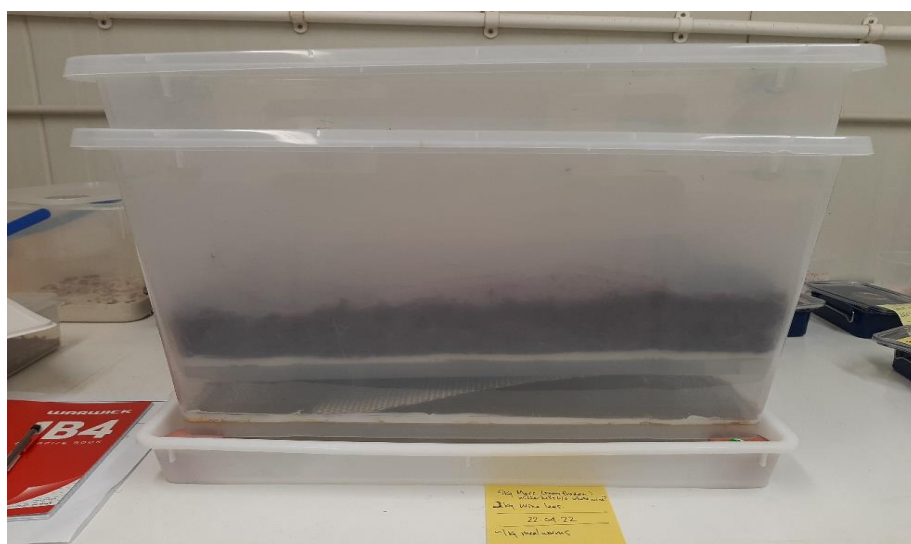
Figure 4. A large experimental feeding box (prototype 2) to monitor mealworm ( Tenebrio molitor ) feeding. The feeding box consists of two stacked boxes. The top (inside) box has a large mesh base, allowing the grape seed to be separated. The lower box has a finer mesh, allowing frass to fall through to the tray below. The lower box sits on four rubber stoppers, one in each corner.
