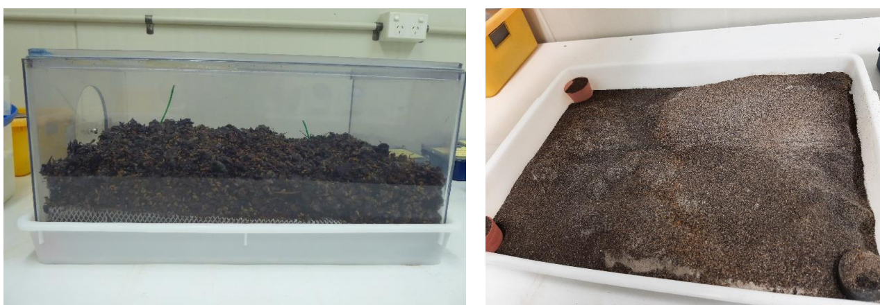
Figure 3. A large experimental feeding box (prototype 1) to monitor mealworm ( Tenebrio molitor ) feeding. The base of the box had two mesh layers. The top mesh layer allowed grape seeds to fall through and collect on top of the second layer. Insect frass was able to fall through both mesh layers into the white plastic tray. In the left image, the box has been filled with grape marc, and on the right is the separated mealworm frass in the white tray after feeding on a combination of grape marc and flour.
