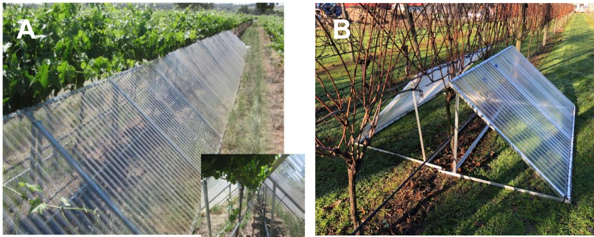
Figure 1. Passive temperature elevation frame (PTEF) systems for simulating warmer growing season temperatures; (A) image taken from Sadras and Soar (2009), (B) two locally developed framed sub-units forming part of the PTEF deployed in the Nelson Marlborough Institute of Technology research vineyard during 2021–22.
