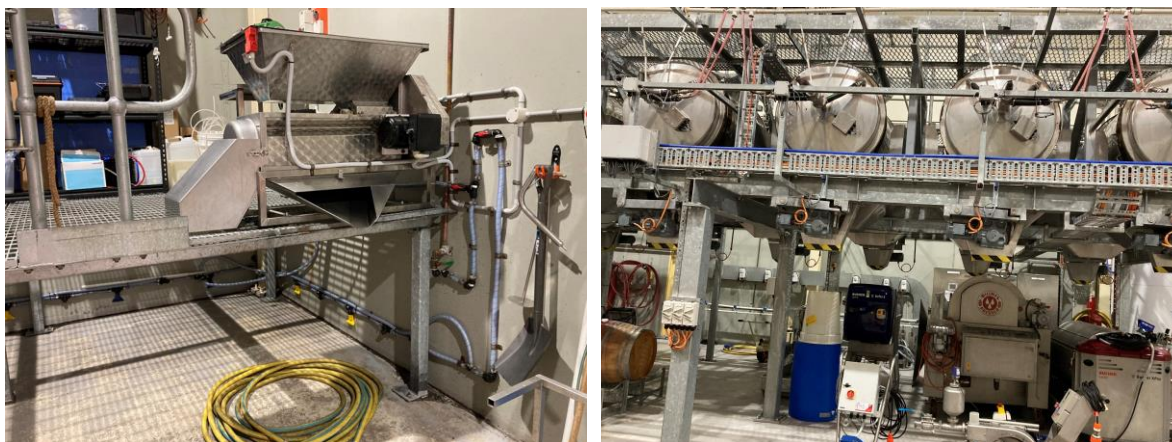
Figure 5. Australian Wine Research Institute (AWRI) research winery. Small-scale crusher destemmer (left) and rotating fermenters on top with press below (right).
