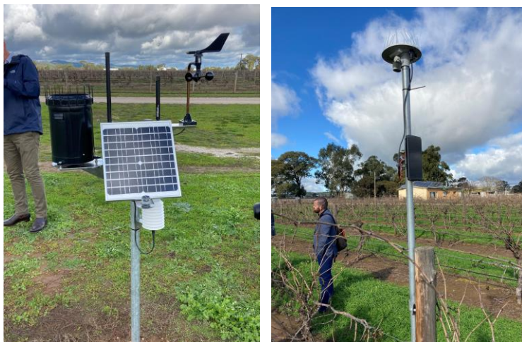
Figure 3. Examples of a micro weather station (left) and soil moisture probe (right) for real-time irrigation monitoring.
