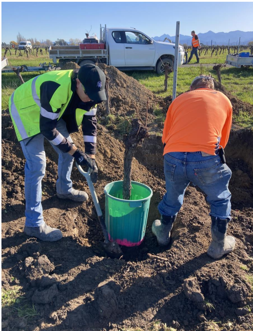
Figure 6. Third vine and soil extraction. During this extraction, a rubbish bin that had the bottom cut out was placed on the soil surface and the soil around it dug out by hand. When 10 cm had been dug out, the top of the bin was pushed down, protecting the core of soil around the roots.
