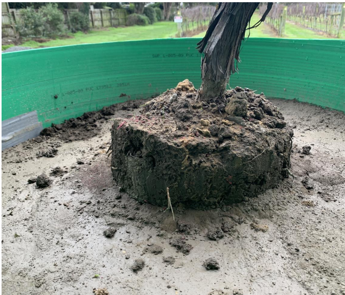
Figure 10. During the filling of the prototype pot with layers of packed silt, sensor tubes and the transplanted vine were inserted into the pot leaving space for a final layer of topsoil and turf or other cover crop to be added.
