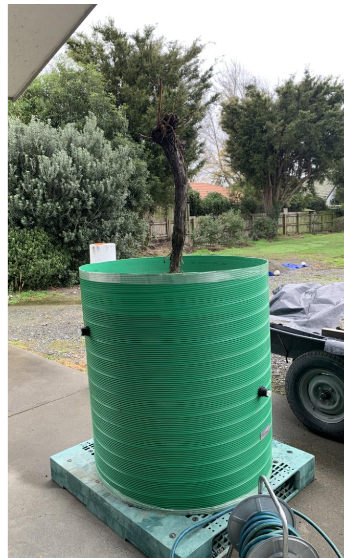
Figure 11. The transplanted vine is now in the prototype pot with sensor service points and on a pallet ready for experimentation.
