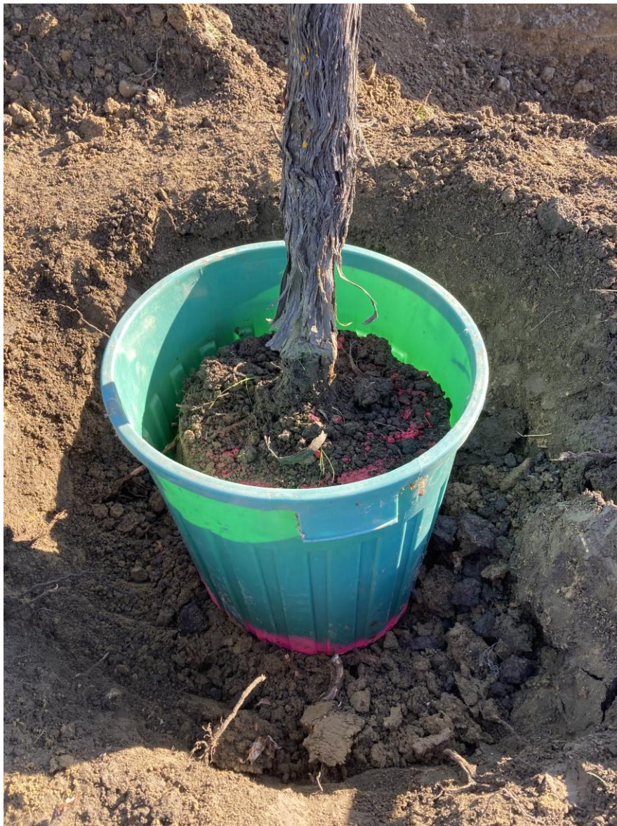
Figure 8. When the bin was covering 50 cm depth of roots and soil the pot was undercut by hand so the core could be removed.
