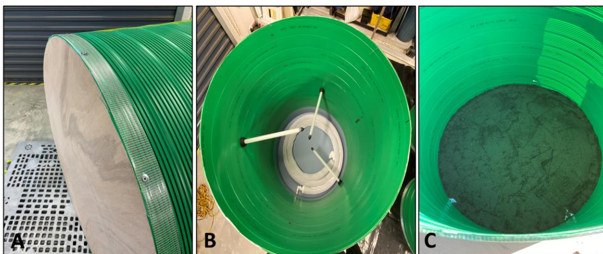
Figure 3. Prototype grapevine planter construction showing, A) attachment of 20-mm marine plywood base to Acrowtube, B) grey/light blue acrylic polyurethane waterproofing membrane, drainage system and placement of soil moisture sensor access tubes, and C) levelled and lightly compacted sand drainage layer.
