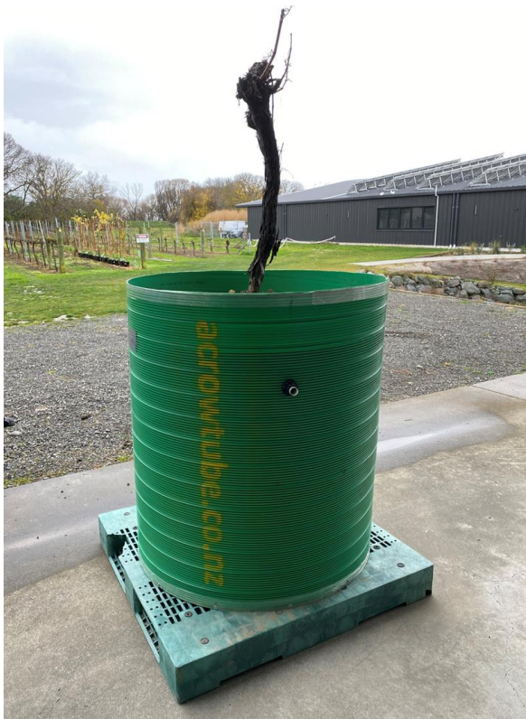
Figure 5. Finished 1.04-m 3 prototype grapevine planter containing leachate drainage and collection system, reconstituted, layered and compacted silt subsoil, various instrument sensing access tubes and intact transplanted mature vine from a commercial Marlborough vineyard.
