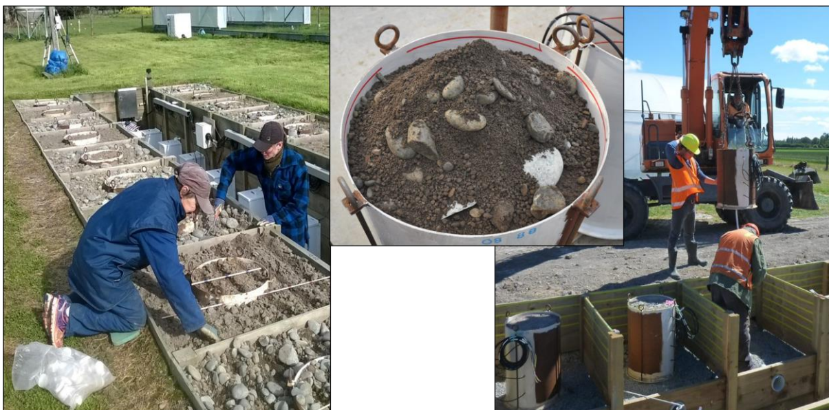
Figure 1. Images of the Plant & Food Research Lincoln 'mini-lysimeter' platform developed in the early 2010s for studying root function and water extraction in shallower-rooted pasture and arable crop stands.
