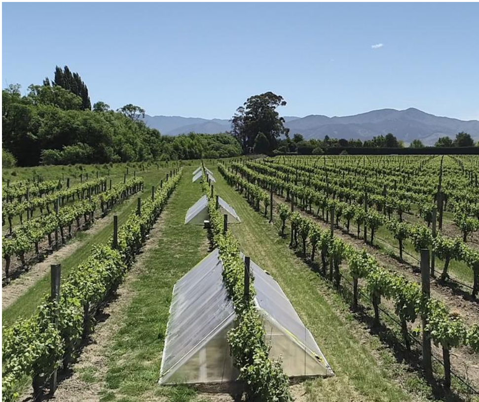
Figure 2. Aerial drone image (looking North) of the single row replicated trial located at the Marlborough Research Centre (MRC) Rowley Research vineyard, showing the arrangement of elevated temperature (PTEF) treatment plots, with ambient temperature control plots interspersed between. For scale, the length of plots (one complete PTEF system) was 7.2 m. Image taken on 9 November 2022 and courtesy of Dr Stewart Field, Nelson Marlborough Institute of Technology (NMIT).
