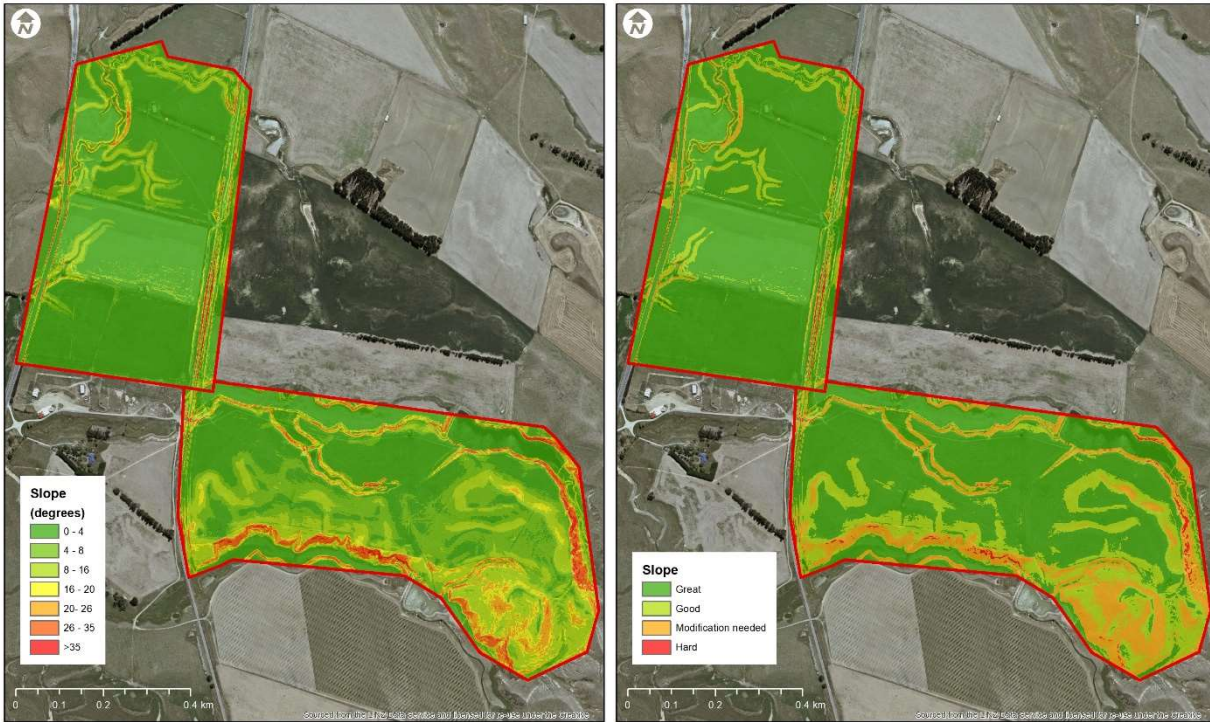
Figure 3-2: Slope map for Survey Areas 1 & 2 (left) and a classification based on ease with which large irrigation infrastructure could be used.
