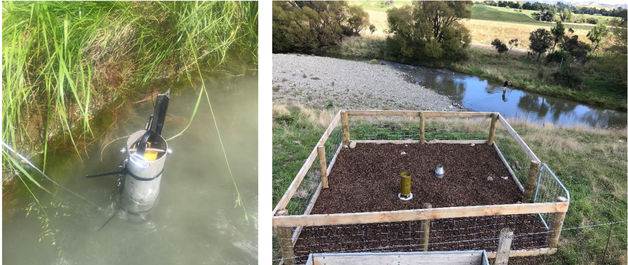
Figure 2-2: Turbidity sensor (left) and hydrometric station (right) at Corrie Downs. The recorder housing and PumpPro are situated on the left bank and the Exo3 is installed at the external staff gauge on the right bank.
