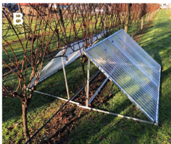
Above: Passive temperature elevation frame (PTEF) systems for simulating warmer growing season temperatures; (A) image taken from Sadras and Soar (2009), (B) two locally developed framed sub-units forming part of the PTEF deployed in the Nelson Marlborough Institute of Technology research vineyard during 2021-22.
