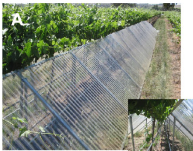
Above: Passive temperature elevation frame (PTEF) systems for simulating warmer growing season temperatures; (A) image taken from Sadras and Soar (2009), (B) two locally developed framed sub-units forming part of the PTEF deployed in the Nelson Marlborough Institute of Technology research vineyard during 2021-22.
