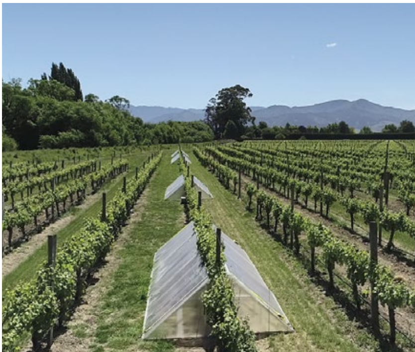
Above: Drone image (looking North) of the single row replicated Climate Change Simulation trial located at the Marlborough Research Centre (MRC) Rowley Research vineyard during season 2022–23. Shown is the arrangement of elevated temperature (PTEF) treatment plots, with ambient temperature control plots interspersed. For scale, the length of plots (one complete PTEF system) was 7.2 m. Image taken on 9 November 2022 and courtesy of Dr Stewart Field, NMIT Te Pūkenga.
